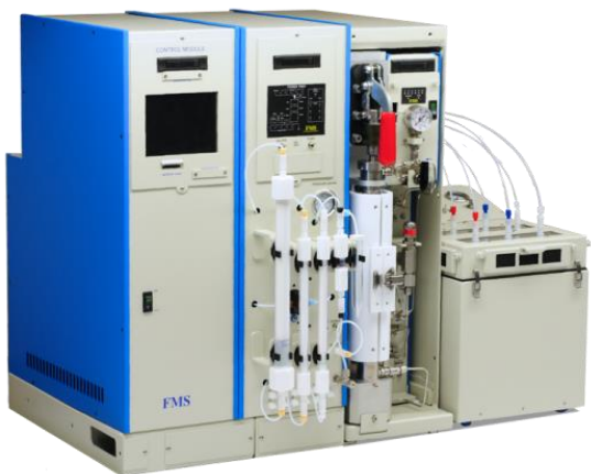
PLE™ Pressurized Liquid Extraction Module PowerPrep™ Multi-column Sample Cleanup Module SuperVap™ Evaporation and Solvent Exchange Module
