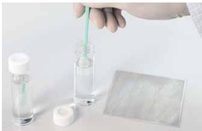
Figure 1a, 1b: Swab sampling on a test specimen, cross-wise in lanes
