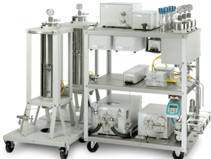
Figure 4: Waters Bio-Botanical Extraction System (BBES). The pumps are on the bottom, 5 L extraction vessels to the left, and three 2 L cyclone separators at the top right.
