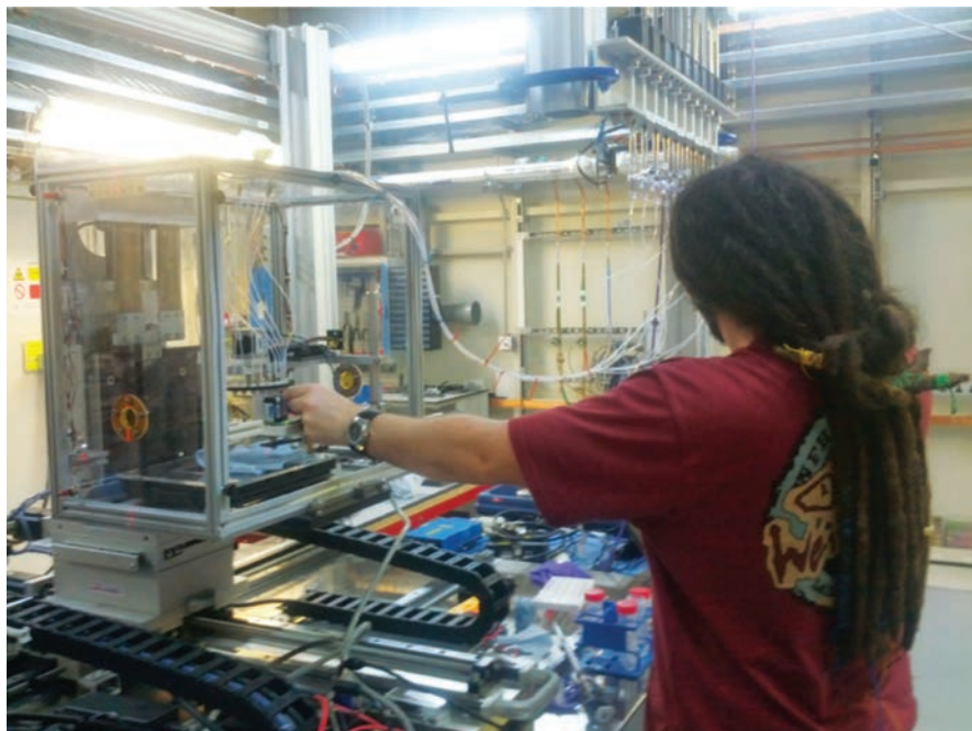
Chris Polin, one of the research team, loading Mjolnir up with a set of samples before they are exposed to Diamond light.
