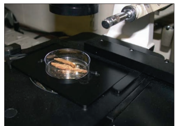
Figure 2. Shows how securely the Petri dish fits into the stage of the inverted microscope.
