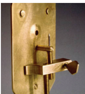
Figure 2. A representation of Van Leeuwenhoek's first microscope
