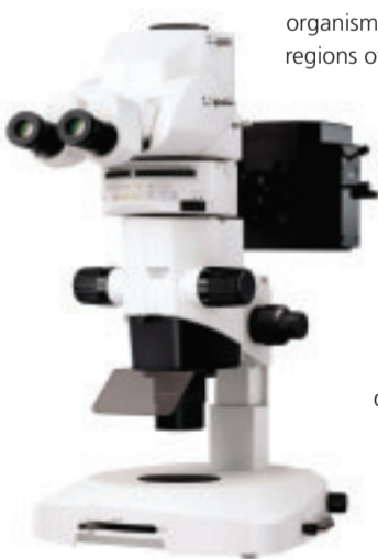
Figure 2: The Olympus MVX10 macro zoom microscope
