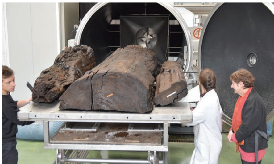
Drying process carried out inside the apparatus for large-scale lyophilisation procedure (Credit ARC-Nuclart) somewhere near top of page
