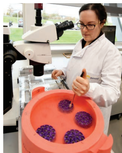
The pins with the mounted crystals are plunged into liquid nitrogen and placed into pucks
