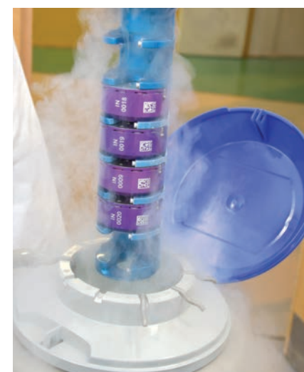
The pucks containing 16 mounted pins each are sealed and placed into storage racks in the liquid nitrogen dewar ready to go to the beamline
