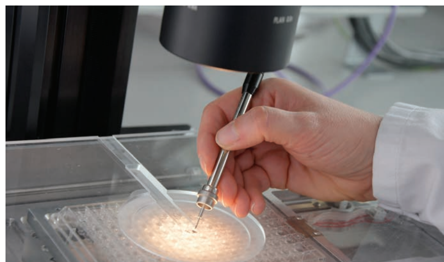
96 well plate of crystals in the crystal shifter ready for fishing crystals with a loop mounted on a pin
