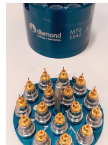
Combipuck base with 123 sample holders and combipuck lid
