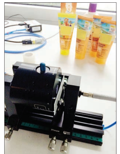
Figure 4. A miniature spectrometer configured for transmission measurements was used to test sunscreen samples applied to surgical tape on microscope slides.
