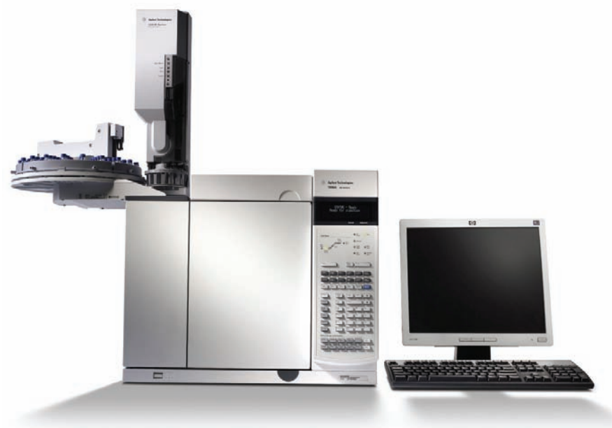
Agilent 7890A GC equipped with automatic liquid sampler
