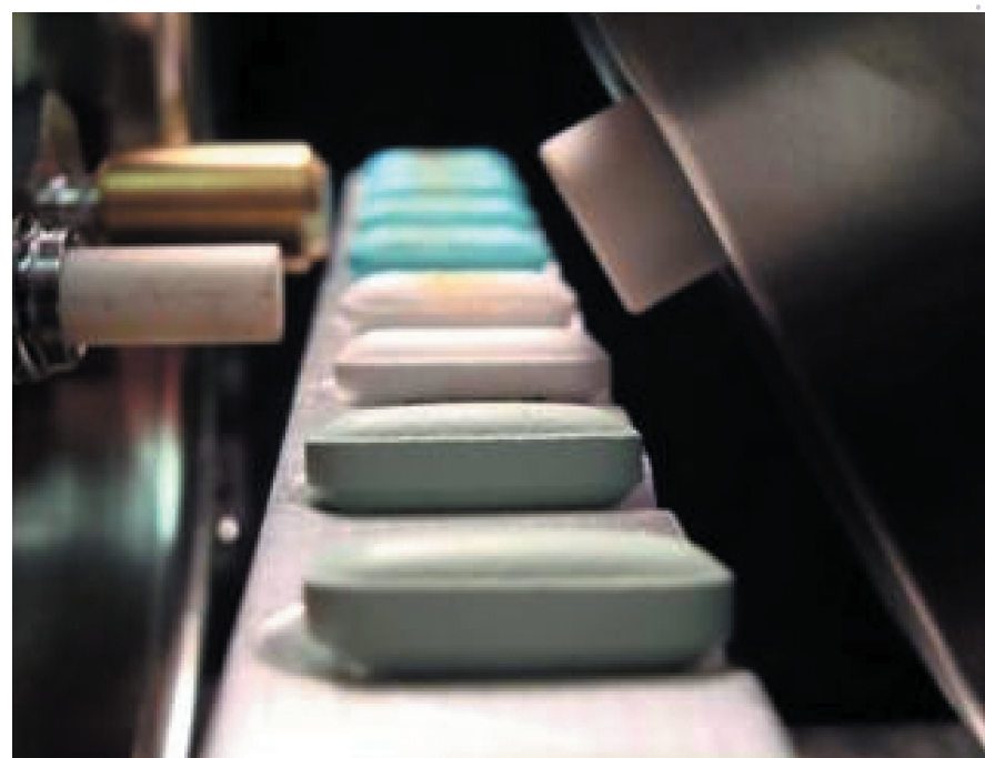
Figure 2. PADI (Plasma assisted photon desorption/ionisation - Courtesy Dave Barrett, University of Nottingham)
