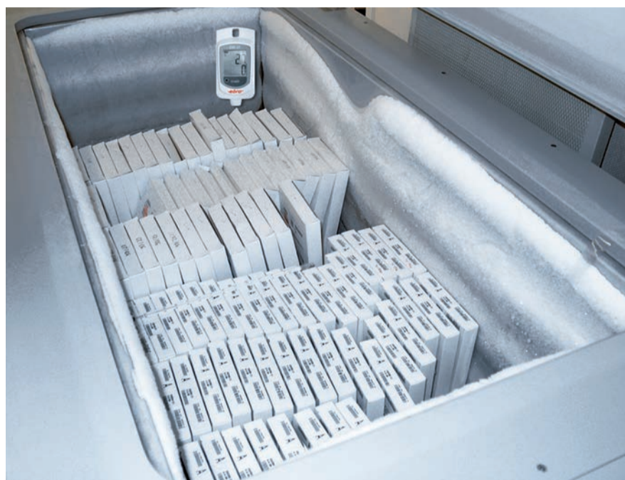
Ebro EBI 25 Wireless Temperature Data Logger monitors vaccines in cold storage
