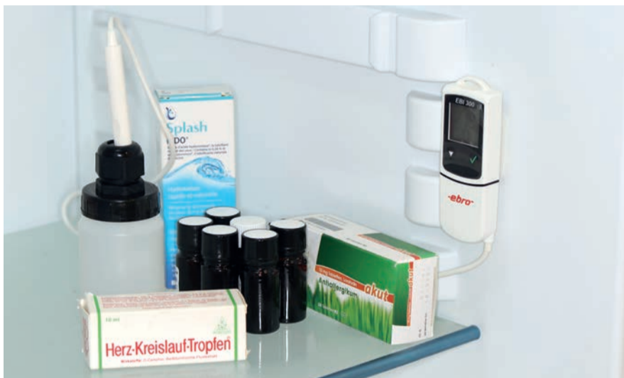
Ebro EBI 300 USB Data Logger monitors the temperature and/or humidity during transport and storage of sensitive goods like medicine, food, serums etc.
