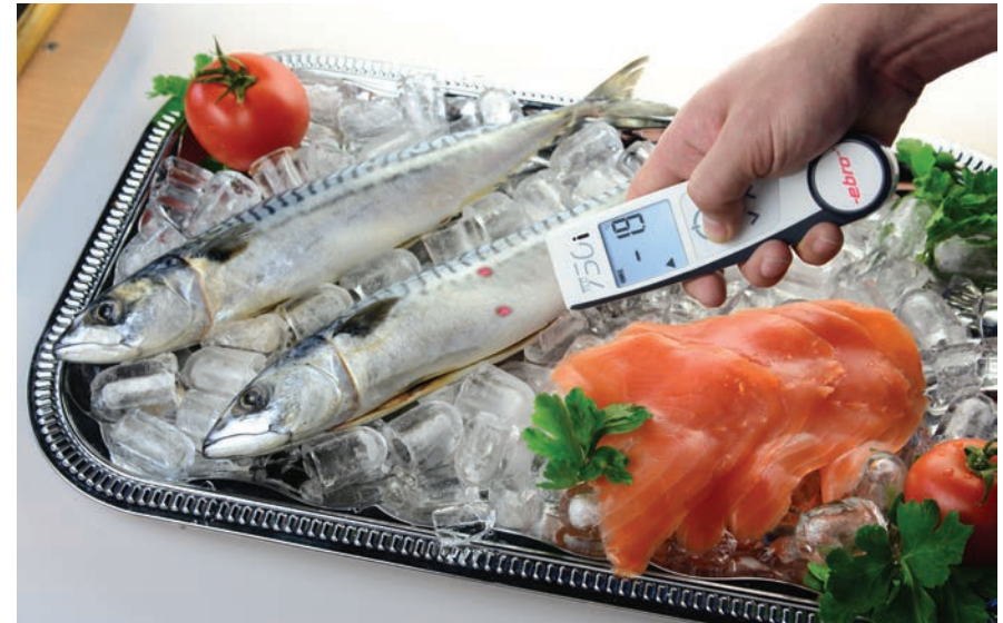
Figure 3: The TLC 750i monitoring the temperatures of fish in market shelves which if not properly controlled can contribute to growth of microorganism and generate histamine levels, both constituting to food safety issues.
