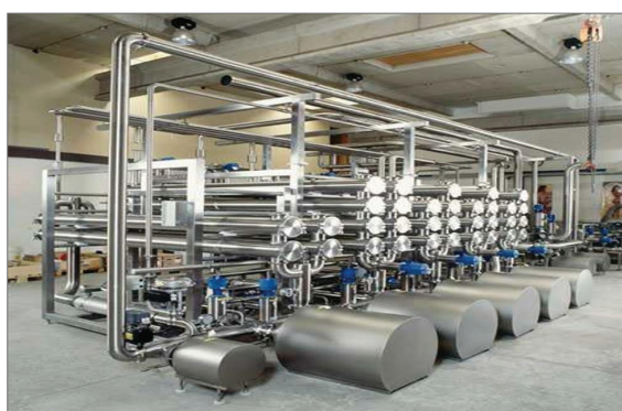
Figure 1. A high efficiency ultrafiltration system (Courtesy of GEA Process Engineering)
