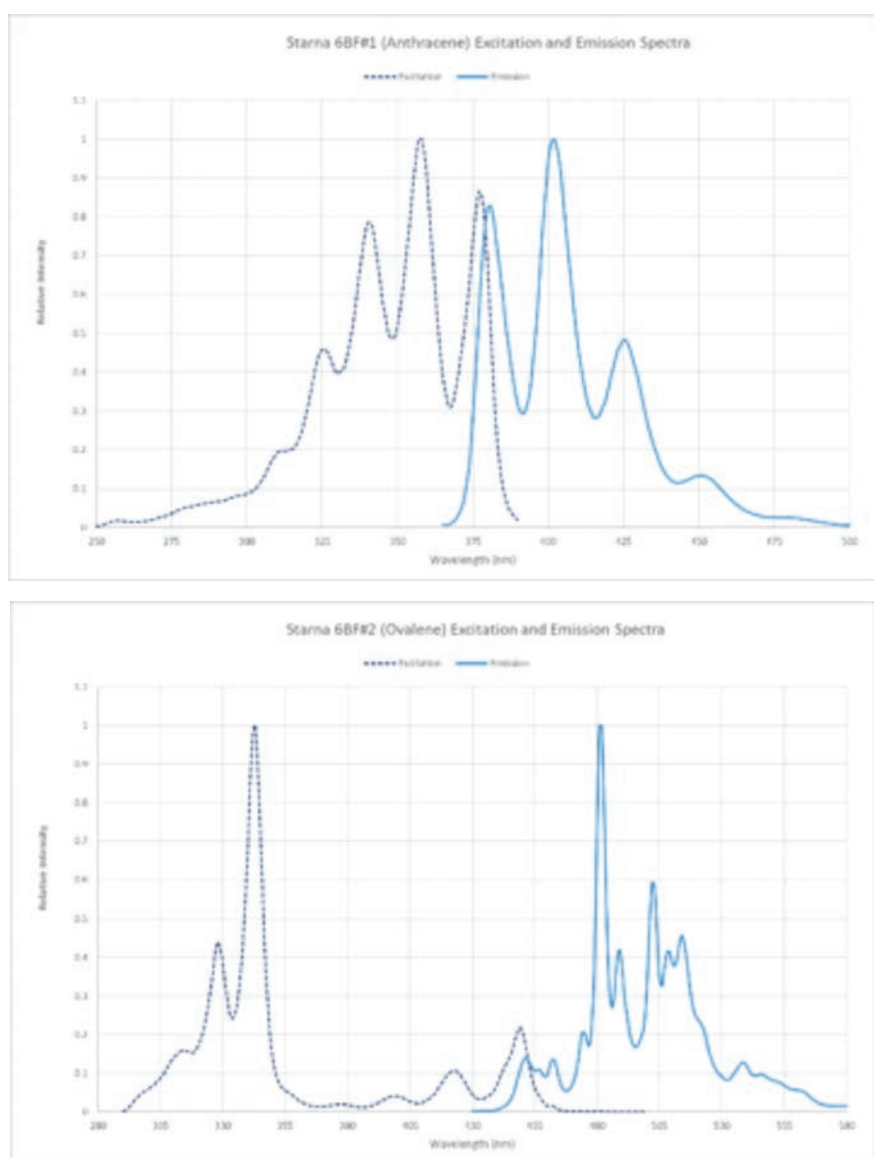
Figure 2. Fluorescence Spectra of Anthracene and Ovalene doped PMMA blocks
