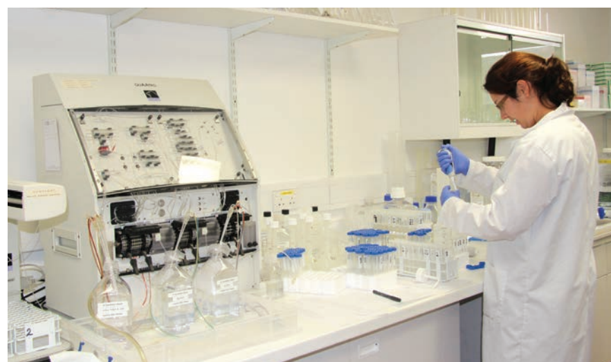
The QuAAtro 39 SFA is the workhorse of the NOC laboratory for micro level nutrients
