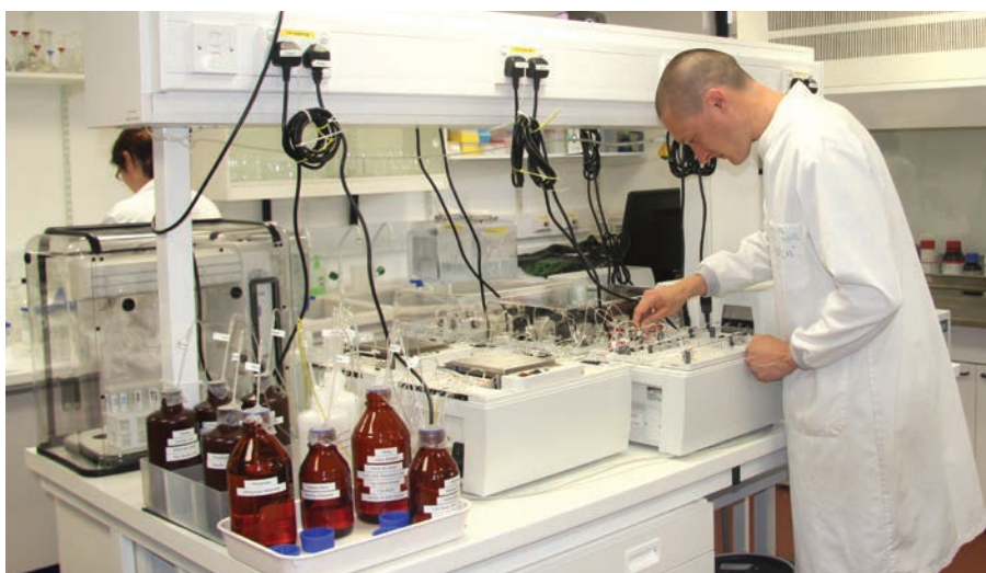
The SEAL AA3 Segmented Flow Analyser is operated in the onshore lab and aboard ocean-going research vessels
