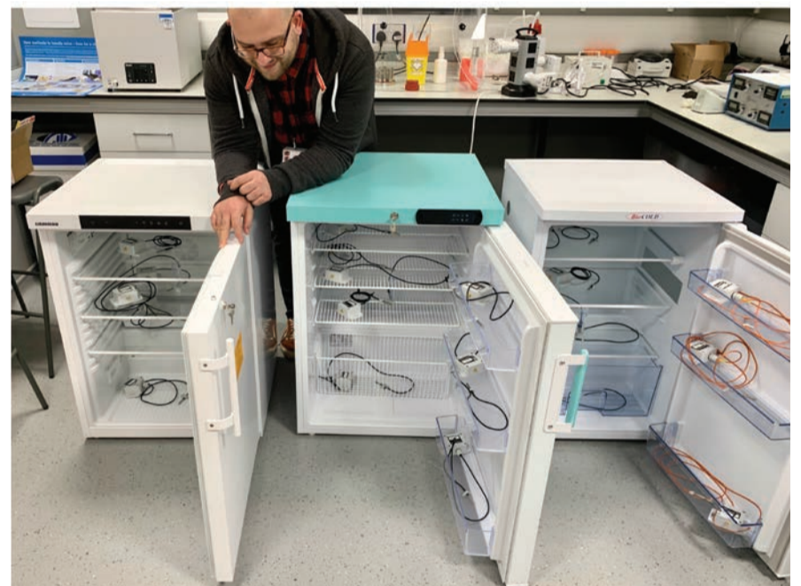
Figure 2. Each fridge with a temperature probe in each compartment together with a temperature probe placed in glycol at the centre most point to represent a sample. Dan Smith from the University of Birmingham holding open the Liebherr door which is self-closing.
