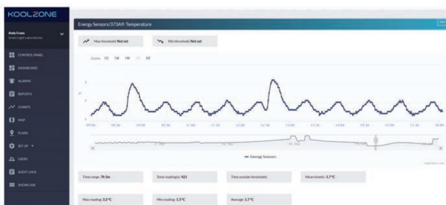
Figure 4. Lec door opening data from the sample probe. Door openings occurred at 9.39am and 12.28pm.
