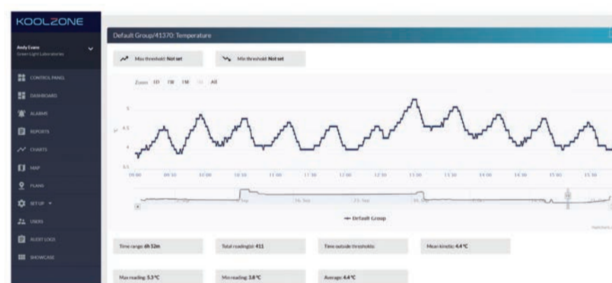
Figure 5. Biocold door opening data from the sample probe. Door openings occurred at 9.37am and 12.31pm.
