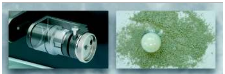
Figure 2. After a few minutes of grinding, the sample shows a fineness of 100 microns and less.
