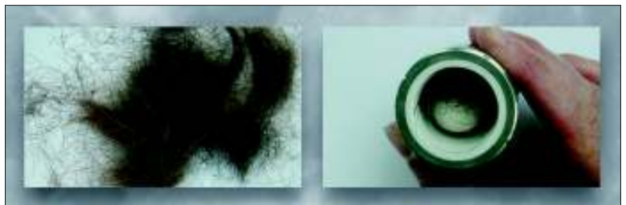
Figure 1. The hair sample and a grinding ball are filled into the grinding jar.
