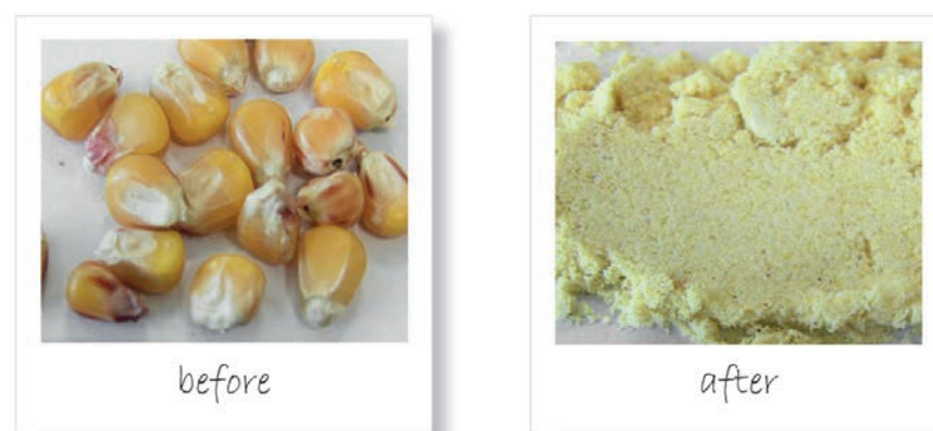
Figure 3: corn before and after homogenisation in a rotor mill.
