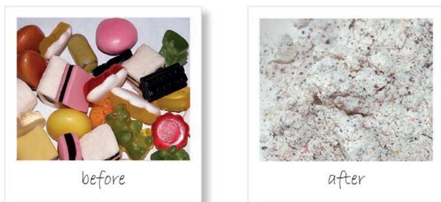
Figure 4: fruit gum before and after grinding with dry ice in a knife mill.
