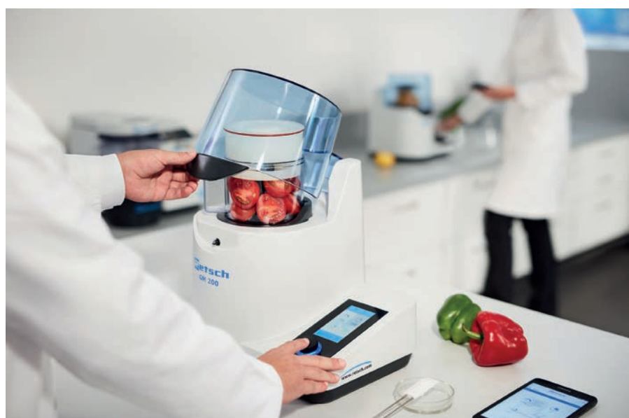
Figure 1: Knife Mill GRINDOMIX GM 200.
