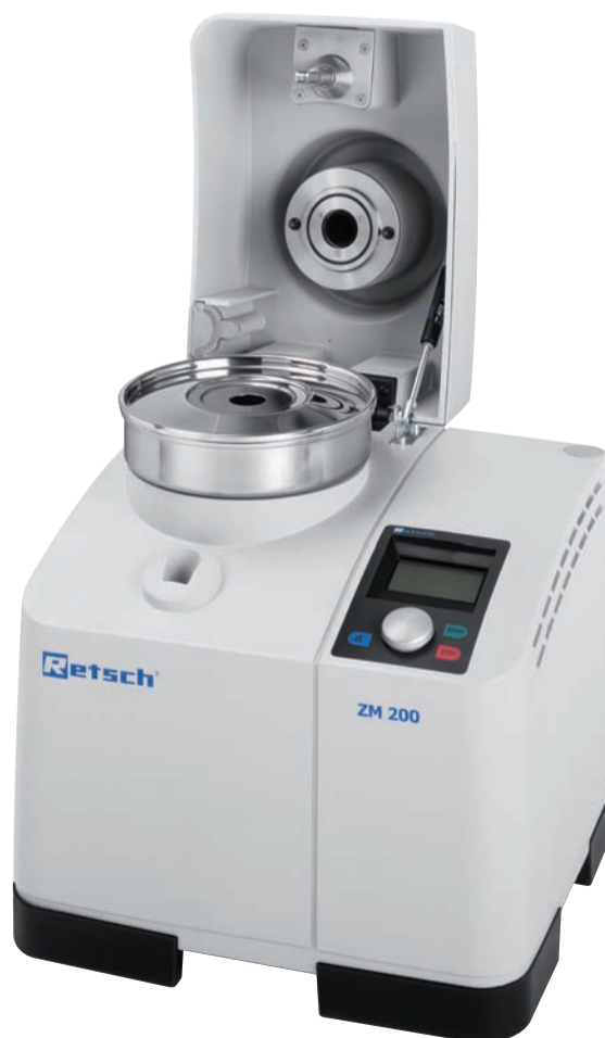
Figure 1. Retsch ZM 200 Ultra Centrifugal Mill for rapid grinding of rice, feed size 3-8mm, down to a size range of 60 – 100µm in minutes
