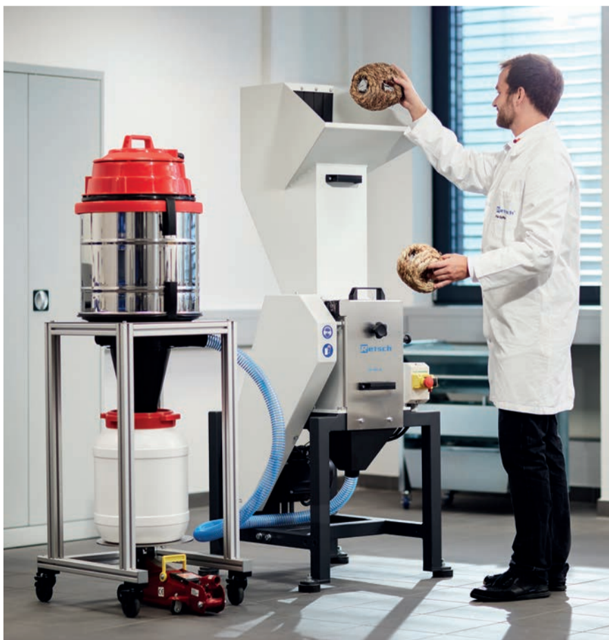
Figure 1: Cutting Mill SM 400 with cyclone-suction combination.
