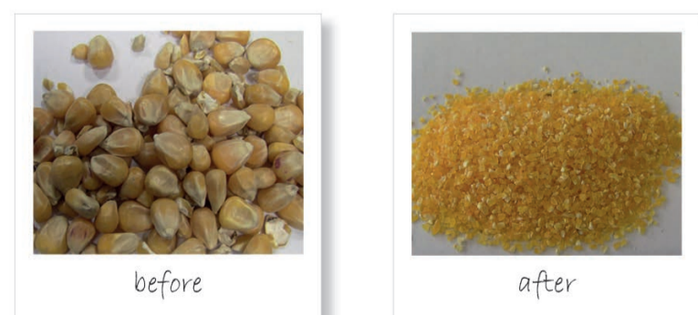
Figure 3: Maize kernels before and after size reduction in the SM 400.
