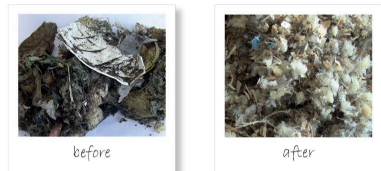
Figure 2: Refuse-derived fuel sample before and after size reduction in the SM 400.
