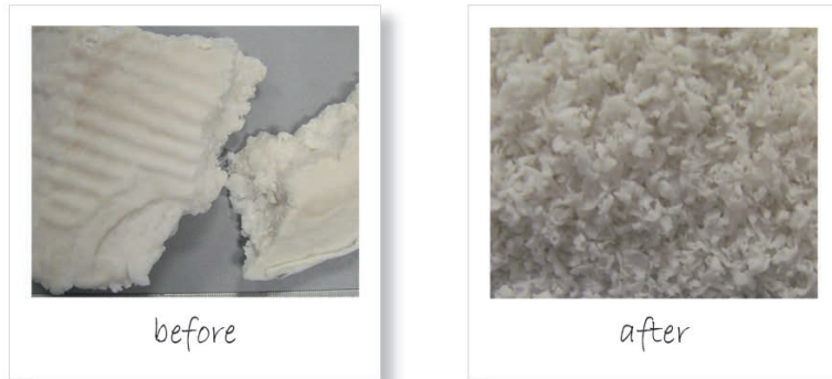
Figure 4: Cellulose pressed fibre mat before and after grinding in the SM 400.
