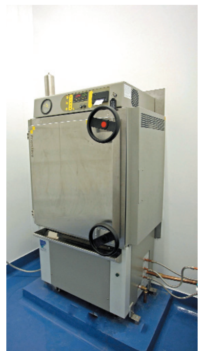
Figure 3: The service end showing the effluent retention filter protruding from the top and the TACTROL® data print-out record on the right of the fascia panel.
