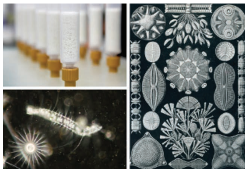
Figure 2. Diatomaceous earth (DE) is composed of naturally occurring silica-based mineral made from fossilised diatoms, a class of hard-shelled algae found in seas and oceans. Its small pore size and high surface area makes it the ideal material for absorption of aqueous solutions.
