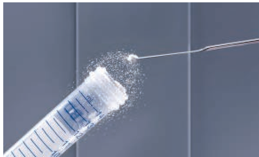
Figure 1. 'Jumping' powder during the weighing-in step caused by electrostatic charges.
