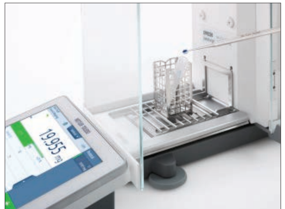
Figure 5. Weighing with an ErgoClip, a small metal basket, which acts as a tare vessel holder and shields the vessel from electrostatic charges.
