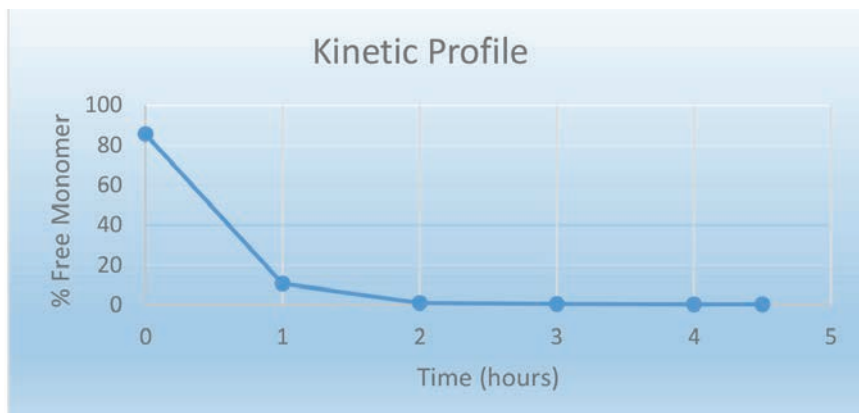
Figure 7: Reduction in monomer peak height at 700-740\text{cm}^{-1} v's time follows closely the kinetic profile of the reaction as shown above and in Table 1.
