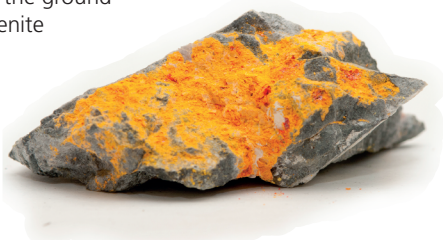
Figure 2. Arsenic is not usually to be found in its pure form in nature. One of the compounds frequently encountered is realgar ( \text{As}_4\text{S}_4 ), here seen on a substrate of stibnite and granite .
