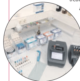
Figure 6. As well as COD, LANGE cuvette tests determine NH 4 , AOX, NO 3 , NO 2 , PO 4 , N tot in leachate
