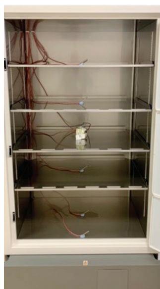
Figure 1. The F740hi with probes positioned at the centre of each shelf. Furthermore, additional probes were positioned at the back of the top compartment (compartment 1) and the front of the bottom compartment (compartment 5). Compartment 3, the middle compartment, had its probes positioned to be exactly at the middle point of the cabinet.
