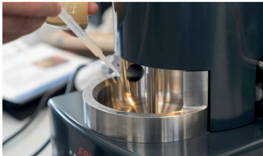
Figure 2: Pipetting the pre-dispersed sample into the wet measuring unit of the A-22 NeXT,
