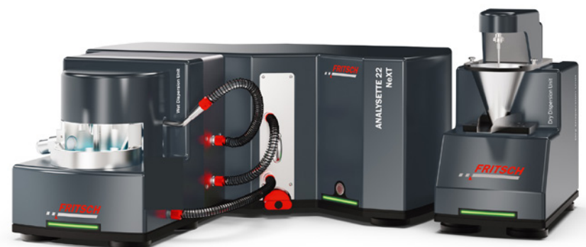
A-22 NeXT with wet and dry dispersion unit - The Laser Particle Sizer for wet and dry dispersion.
