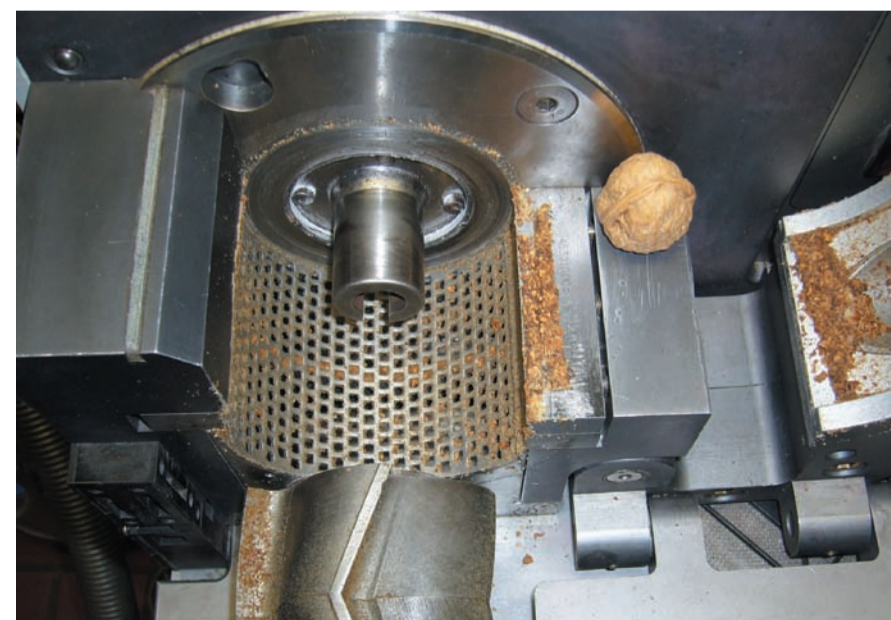
Figure 3. The glance into the open grinding chamber shows an optimal throughput of the walnuts
