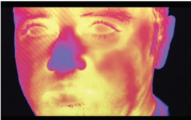
The ISMS thermal camera monitors facial temperature modulation of the crew while performing typical pilot tasks.
