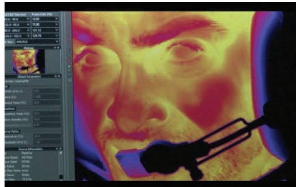
The ISMS thermal camera monitors facial temperature modulation of the crew while performing typical pilot tasks.
