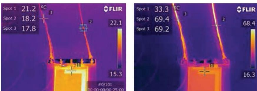
Cables with a low current rating are put to the test. If approved for use, these cables will contribute to keeping the weight of the car low.
