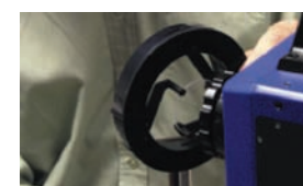
To visualise the escaping CO 2 the researchers used an external band-pass filter.
