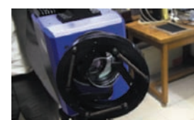
The external band-pass filter is centred on the CO 2 emission peak.
