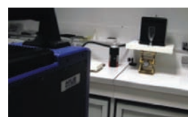
The SC7000 operates at a bandwidth of 3 to 5 μm, the external filter narrows it down to exactly 4.245 μm.
