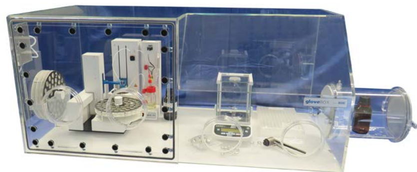
Figure 9: Arrangement of the Karl Fischer titrator and the analytical balance in a customised glove box with four glove ports
