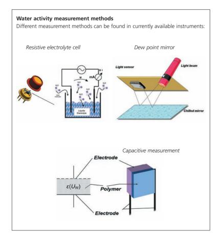
Some measuring sensors have in-built calibration data memory at a number of points across the range or aw. The accuracy of available instruments in the market is  $\pm$ /- 0.003 aw
