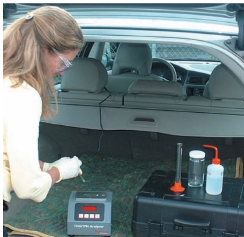
On Site FOG Measurement
