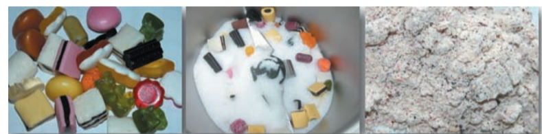
Figure 2. Grinding a wine gum mixture with dry ice in the GM 300
