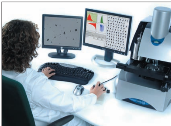
Figure 1. The Morphologi G3 automated particle characterisation system combines light microscopy and image analysis
