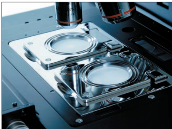
Figure 2. A glassless sample carrier allows two filters to be mounted at once, for successive analyses without manual intervention (Morphologi G3)
