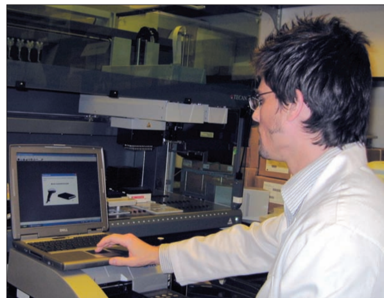
Figure 1. Xenotech Research Scientist of R&D/Method Validation of Laboratory Automation, Robert T. Grbac, using the Artel MVS® to measure the accuracy and precision of his automated liquid handler.
