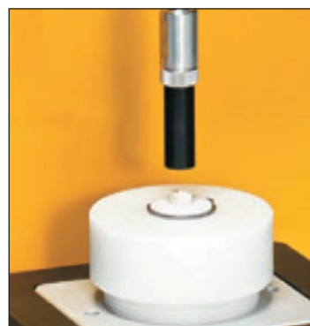
Figure 9a. Dough Stickiness Fixture is Standard Test for Measuring Dough Stickiness which is an Important Parameter for Processing Raw Dough.
