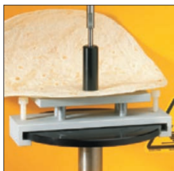
Figure 2. Junior Punch Assembly for Measuring Hardness
