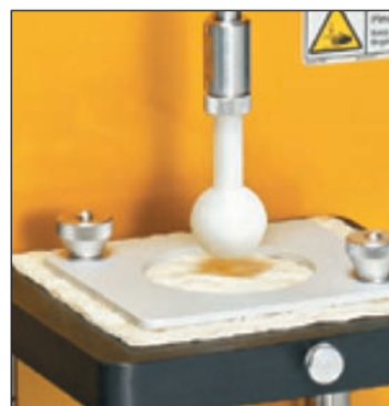
Figure 9c. Dough Extensibility Fixture for Holding Sheet of Raw Dough or Flat Bread such as Tortilla. Biaxial Test Force is Applied by Spherical Probe. Test Measures Force and Distance as Sample is Stretched to Breaking Point.
