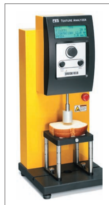
Figure 7. CT3 Texture Analyser Tests Bread
