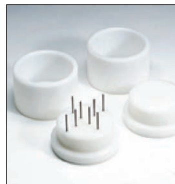
Figure 9b. Standard Dough Post Set for Preparing Dough Samples and Measuring Dough Firmness.
