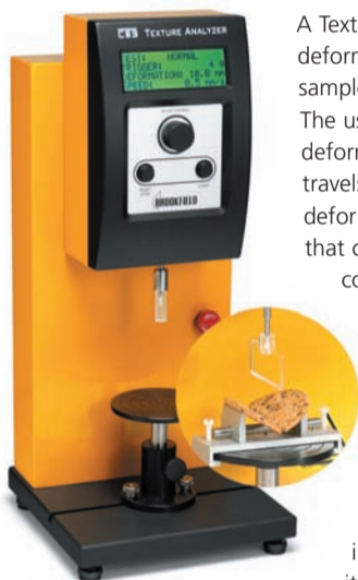
Figure 1. Brookfield CT3 Texture Analyser Performs Snap Test on Cracker
