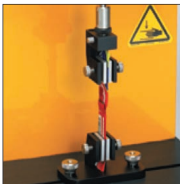
Figure 3. Dual Grip Assembly for Tension Test
