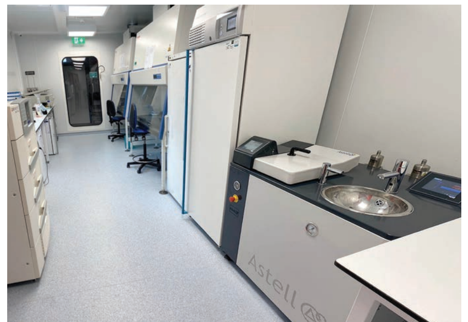
The FarmLab Laboratory features an AstellBio Sink & Autoclave Combo thermal sterilisation station.
