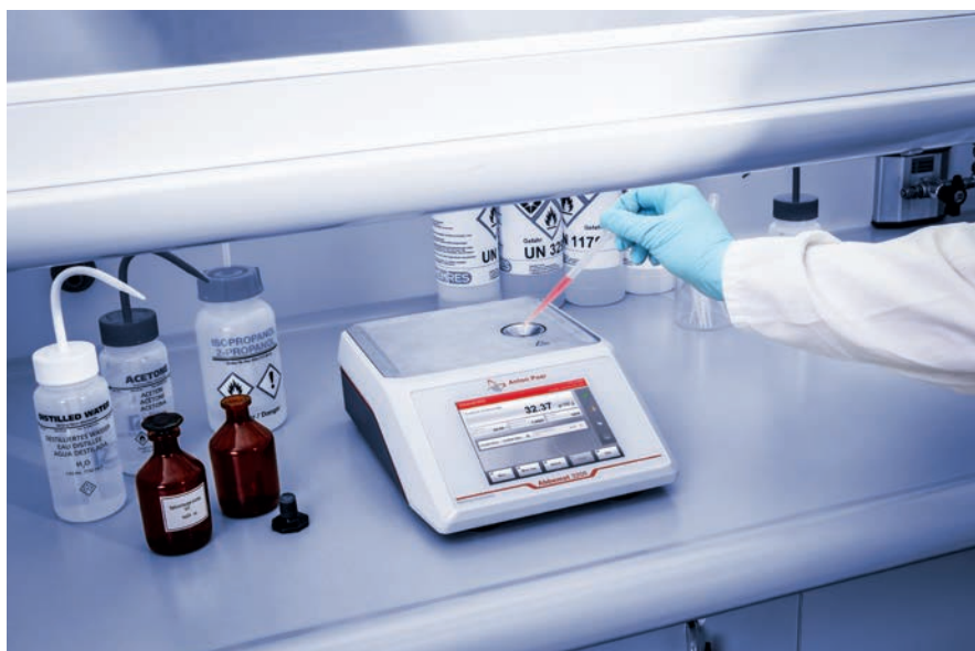
Figure 1: Abbemat refractometers from Anton Paar are able to measure the concentration of acids and bases within seconds from just a drop of sample. They are a very economical alternative to conventionally used titrators.
