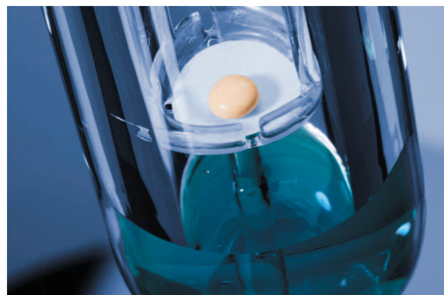
Image 3. Beside standard acid digestion, unique applications like microwave-induced oxygen combustion (MIC) can be carried out in Multiwave PRO.
