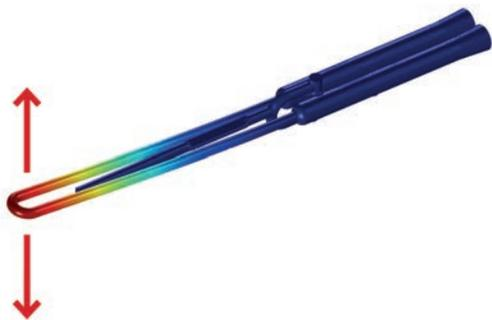
Figure 3a. Working principle of a Y-oscillator.
