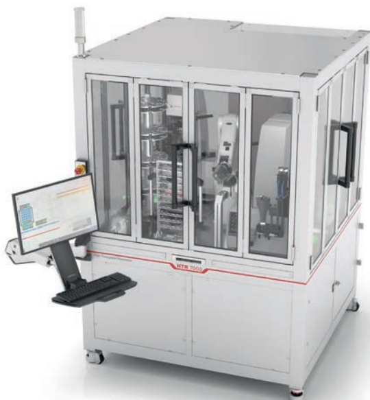
Figure 4: The HTR 7000: Fully Automated Rheometer for CC, CP or PP measurements with the automatic trimming tool, a robotic arm, and storage racks for sample discs and sets of measurement geometries, option for sample preparation and fully cleaning the upper and lower measurement geometries.
