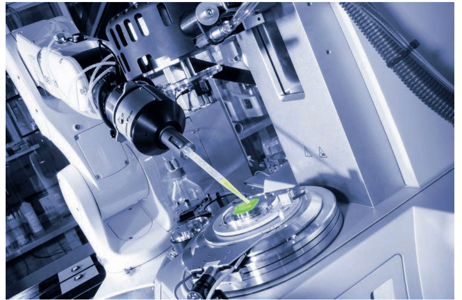
Figure 5: Attaching the cone, dispensing the sample, and loading in the cleaning unit for a high-throughput rheometer with a six-axis robotic arm and a rheometer equipped with a Peltier temperature device and cone-plate geometries.
