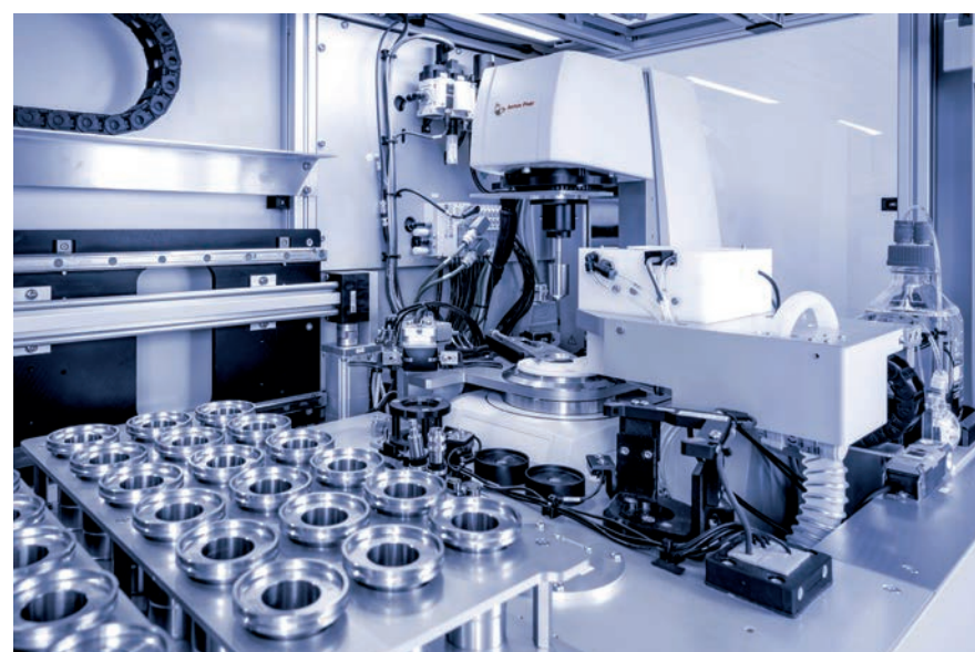
Figure 2: Inside the HTR 3000, storage racks on the left, automated cleaning on the right, MCR 302e in the back.
