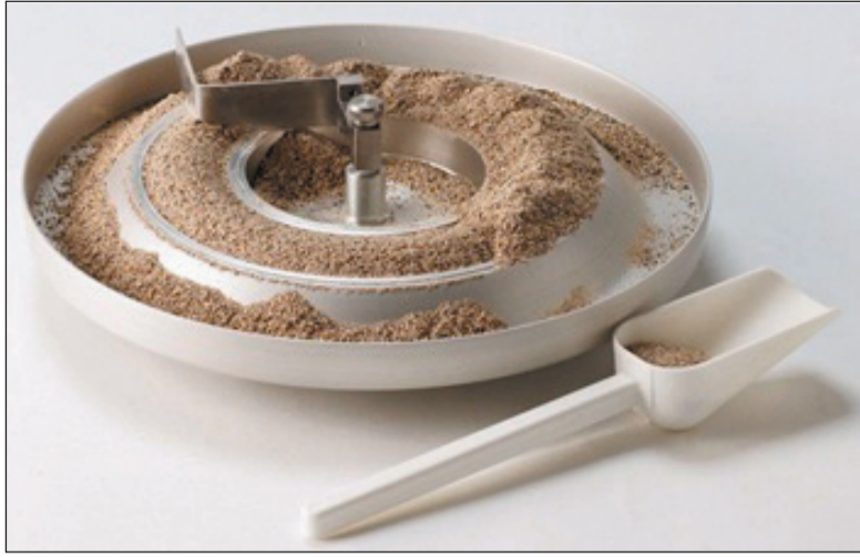
Figure 5: Sample Preparation of Powder in Shear Cell
