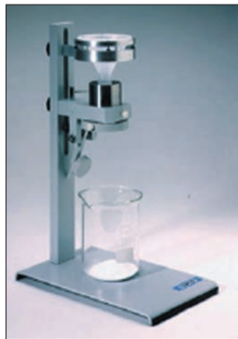
Figure 1. Flow Cup Gives Go/No-go Indication for Loosely Consolidated Powder
