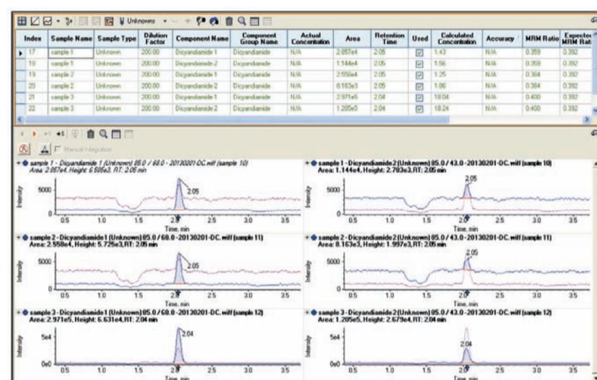
Figure 6. Milk samples tested positive for dicyandiamide, the 'Multicomponent' query was used to automatically calculate MRM ratios for compound identification
