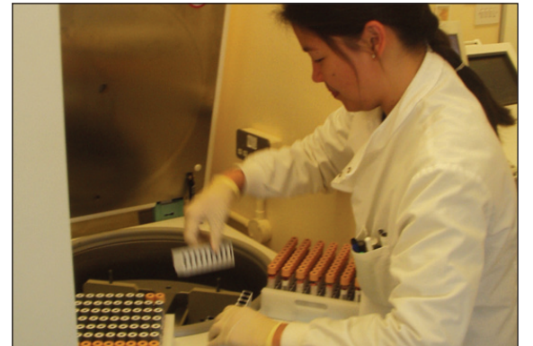
Figure 2. Centrifugation is performed separately since built-in centrifugation was felt to be a limiting step in creating a high volume test system
