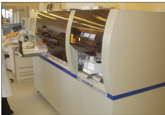
Figure 3. Pre- and post-analytical stages are automated using the OLA2500, which sorts sample tubes according to test requests and decaps and aliquots as required
